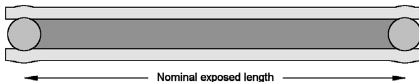
Figure 25 Gravimetric permeation testing of breathing hose.
