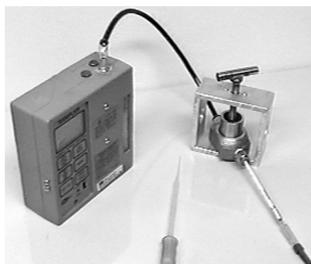
Figure 16 Using a personal sampling pump to measure glove permeation
